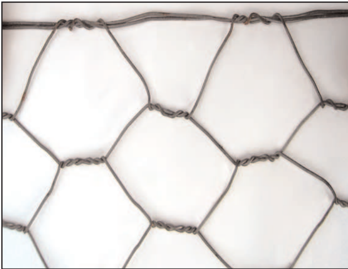
Figure 2. Enlarged view of chicken wire, showing the weaving of the hexagonal pattern and the selvage along the edge.
