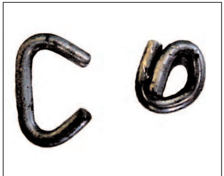
Figure 7. Hog rings opened and closed.
